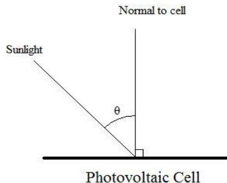
The normal to the cell is perpendicular to the cell's exposed face. The sunlight comes in and strikes the panel at an angle. The angle of the sunlight to the normal is the angle of incidence ( $\theta$ ). Assuming the sunlight is staying at a constant intensity ( $\lambda$ ) the available sunlight to the solar cell for power generation ( $W$ ) can be calculated as:
